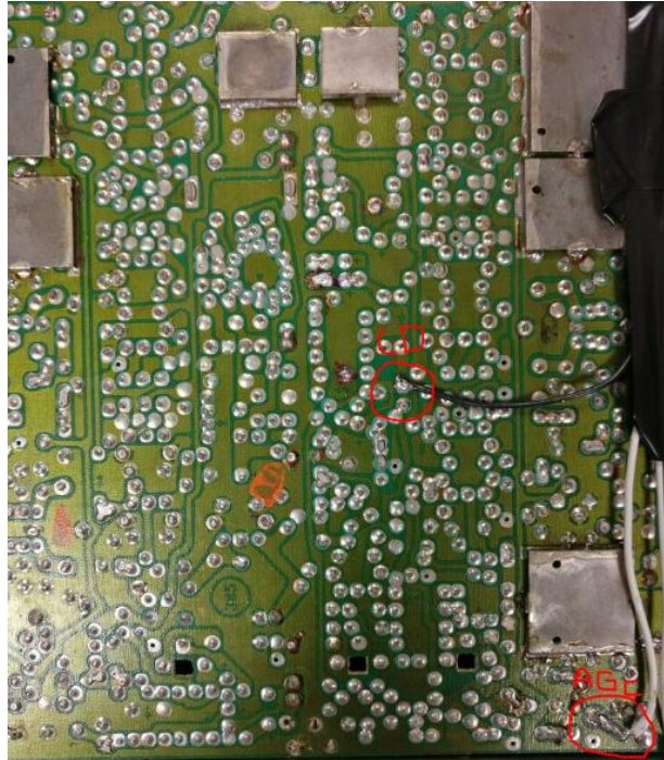
Figure 3.5 Where team tapped into radio for AGC and RX Audio
