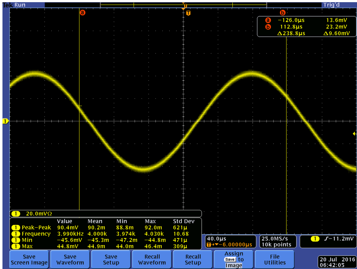
Figure 6.18 RX Audio Input with No Offset
